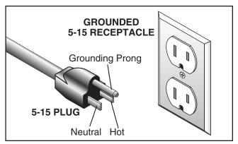
Figure 1. Typical 5-15 plug and receptacle.
